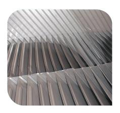
settlers by substituting the projected area for the surface settling area of a conventional settler. Furthermore, with the addition of a sludge thickener to the plate settlers, increased underflow sludge concentration and sludge storage flexibility was also possible.
