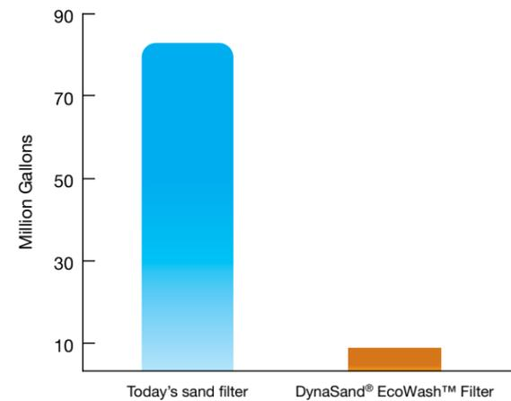
This table gives the annual reject water production for a typical 16 Filter (50 SqFt) – 5.76 MGD capacity facility with standard sand filters as compared to the DynaSand® EcoWash™ Filter.
