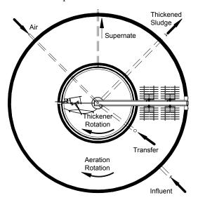
is built within the digestion tank to form the thickener structure. In the digester, flexible membrane diffusers are suspended just inches above
